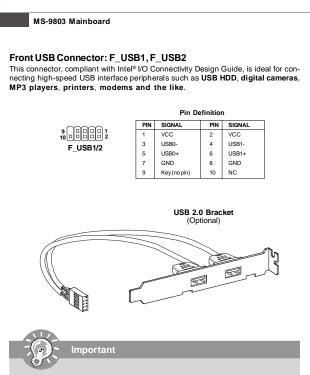
Note that the pins of VCC and GND must be connected correctly to avoid possible damage.
